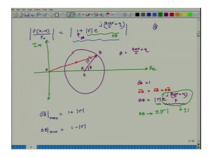
So, in that context we have arrived at this expression modulus of complex amplitude of pressure in the tube equals modulus of 1 plus modulus of gamma times e j 2 omega x over c plus eta (Refer Time: 01:41) this we had equation we had leveled it as equation number 6. Now what we will do is, we will depict this graphically the left side of this equation the right side of this equation in graphical format. So, on a complex plane, let us
