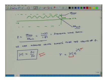
So using the microphone I can find out this ratio OB max and OB min, the ratio of OB max and OB min this ratio is called standing wave ratio it is called standing wave ratio.
