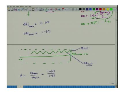
So, what; that means, is that if I plot this is my negative x this is x is equal to 0 excuse me and this is my positive x. So, my tube exists in this direction this is my tube and tube starts from x is equal to 0 at x is equal to 0 it will have some value OB will have some value which will be what 1 plus gamma times e to the power of j eta right. If I am going to plot its value this OB will fluctuate like this and what is going to be the maximum value of this, this is going to be OB max.
