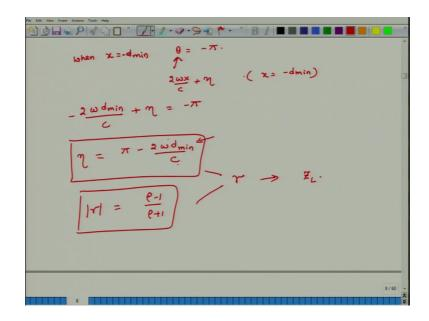
So, what this expression tell that if I can find the value of d min and how do I find the value of d min I just move the microphone, gradually away from the closed end and wherever I find the first minima that is corresponds to the location d min. So, I record that number I know the value of C which is 345 meters per second and I also know what
