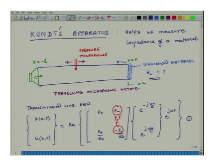
I can actually measure this ratio how can I measure this ratio? I go back to my Kundt's tube and I use this microphone I start sliding it from this location in this direction and wherever I find the pressure to be maximum that will be proportional to OB max and wherever I find pressure to be minimum that will be proportional to OB min.
