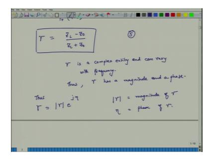
So, Z naught is known Z L if I know then I can calculate gamma and again remember gamma is a complex entity and can vary with frequency because when you take some material, it is impedance or sound absorption properties they change with frequency at certain frequencies it can absorb a lot of sound, at other frequencies it is absorption characteristics are very poor.
