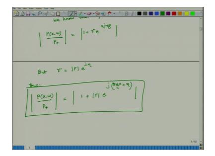
So, I can say that modulus of P x omega divided by P plus equals 1 plus gamma e 2 j omega x over c and finally, we know that that gamma as an amplitude and a phase e times j times eta, thus modulus of P x omega divided by P plus equals modulus of 1 plus modulus of gamma, times e j 2 omega x over c plus eta and the entire thing I have to take a modulus.
