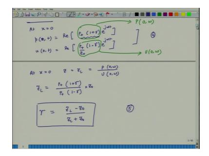
So, once we have done this mathematics then we use the boundary condition. So, what is the boundary condition in this apparatus that at x is equal to 0 the impedance of the system is Z L which we do not know, but it is some number which we do not know and it is Z L. So, this 2 should not be there. So, at x is equal to 0, we will evaluate the pressure and velocity.
