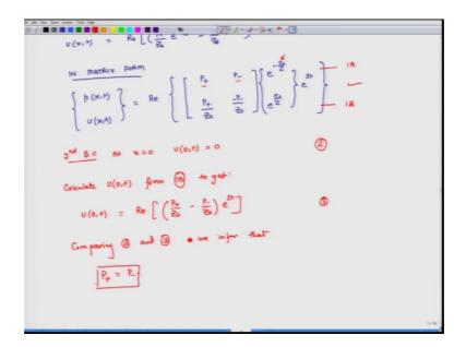
So, we again go back to our transmission line equation and we use the second boundary condition. So, second boundary condition says at x is equal to 0 U of 0 t is equal to 0. So, let us call this equation the first equation has 1 a; this equation is 1 B and this equation as 2.
