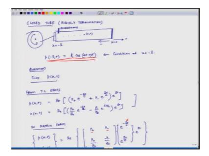
So, we will very quickly go over the problem formulation this is the picture of this tube; one end of the tube where x is equal to minus l, the pressure at the other one end of the tube is P minus l t and that is equal to p 1 cosine omega t plus phi and at the closed end its a closed end. So, it has some physical implication we will come to that just in the moment.
