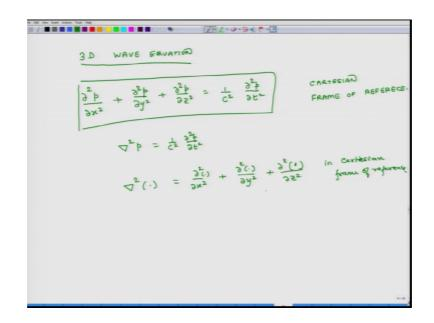
So, when sound is propagating in all the 3 directions then its propagation is governed by 3 d.
