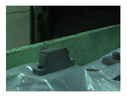
This work piece has 25 mm of width and 160 mm length, discipline machine with this are wheel that is aluminum abrasive wheel.
