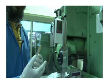
In different machine in treatments did a different like depth of cut and speed combinations we will might observe different Ra values and different force values as well, those would be used to finalize are final setup which gives best mix of this two.
