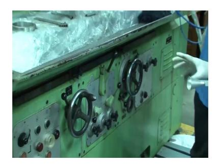
Specifically and the table speed here is we have discreet table speeds available here 2.5 10 15 20 and 25 meter per minute we cannot take continuously we cannot have (Refer Time: 17:34) 2.6 like it meter per minute speed, this is a conventional machine this was a see and see machine.
