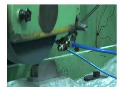
We will we have now fix this attachment here, as to keep this distance specified distance have to the set. Now I have fixed on the compressor and the it is giving see it is giving the spray here the spray rate here is 100 milliliter per hour, is one and in flood, we have of the order of 5 liters per minute is 100 milliliter per hour and see the sprays also the flow it also continuous it is in line flow it will specifically at the point stop work is that like machine is point here.
