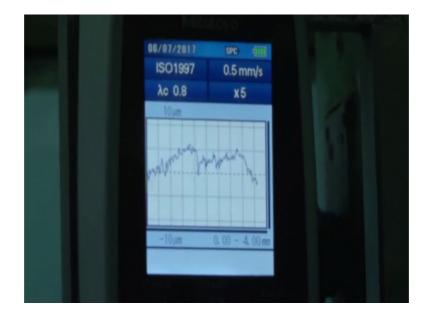
We again doing one experiment to show the graph how the graph is coming here, it has moved 0.8 mm into 5 and this is Ra coming 0.6 micro meter for one sample and we do not only take Ra once we take it is multiple locations here and one location we might do like number of replicates, as to find that their no noise levels here where it is 0.6 micro meter here.
