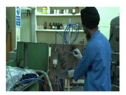
So, for tool like a counter that we made an attachment and we made this close chamber we put a fluid here and these are pressure gauges and air is pressurized to obtain for this is the liquid going out towards the nozzle. This is a air is less pressurizing this one and the liquid and this air pressure towards the nozzle is controlled in such a way that we get continuous flow, continuous like a spray here right, we will fix this attachment and do machining.
