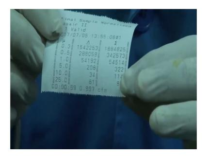
This specific time it has for 59 seconds it has recorded point 0.3, 0.5, 1.0, 5, 10 and 25 micrometer of particles and these are the counts got it thank you.
