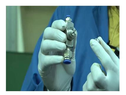
We have already told you that this nozzle this is a single kind of a nozzle here this nozzle has air and liquid inputs here from the 2 valves and we get the like mixture a atomizing here. In this case this is our round cap thus kind of spray would be have; would had be
