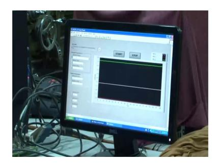
When we do machining these are the force effects we have the force in x, y and z direction, in this case z is our normal force and y is our tangential force x direction we
