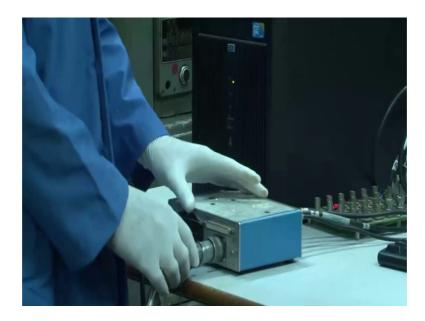
This is lab view software for this is connected here; in this case the force is being transferred into electrical signal that is 1 Newton of force is given 1 volte energy that is for the calibrative we have lab view software here.
