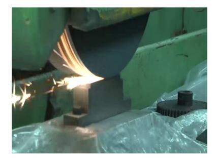
Let us start up; you will start, see he has already given 10 micron feed here we called it feed actually this is the like movement what is up side and he is a now bringing the wheel on this side that is the transfers movement, as the wheel is dressed. This is like we will not run only one here like we will not run only once it will be multiple runs and this is accommended by the wheel manufacture the grinding wheel manufacture he recommends that these are the various parameters.
