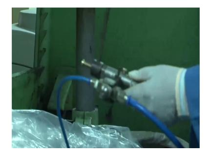
In this, we have this nozzle actually this nozzle is all fixed in our setup excuse me I will show that, we removed just attachment because we have we were to dress the machine this wheel here, this will again fixed is nozzle is kept at a 100 mm distance from our work piece like tool work piece contact work point and this is a setup here.
