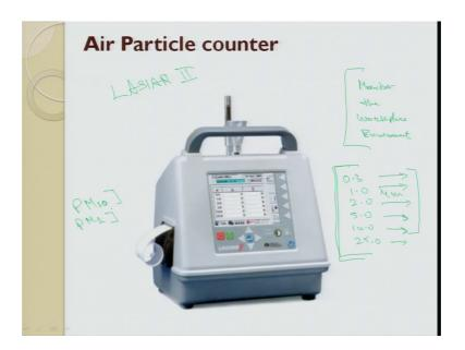
So, the next instrument is air particle counter. This is one of the instruments that we have chosen to monitor the work place environment. Out of the bads that are produced, air emissions are there, noise is there, heat is there; this will count the air particles. What is the size and what is the volume of particles that are present in our machine chop while doing machining.
