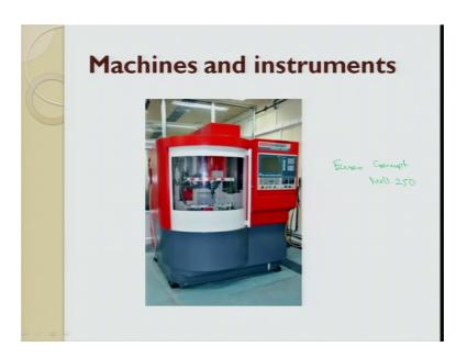
So, also we did milling and drilling differently, but machine that was used was this one this is EMCO Concept Mill 250. I will tell you about the machine when we come to the experiments of drilling and milling.
