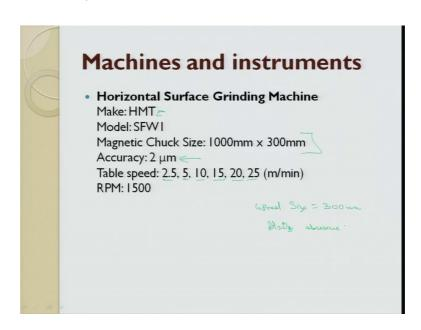
Regarding this machine it is a HMT make machine. The model number is here, the chuck size is here, the accuracy of the machine is 2 micro meter; that is the minimum depth of cut we can give here is 2 micro meter and table speed varies, these are discrete values 2.5, 5, 10, 15, 20 and 25 meter per minute. In RPM that is we also kept RPM same as 1500 RPM here and the wheel size here was 300 mm and it is aluminum abrasive wheel.
