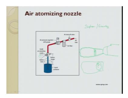
Another system is siphon system; siphon or gravity system. In this case the air pressure is here and there is no pressure, but only through gravity, we have this mist coming up. Also, we have different types of patterns of flow.
