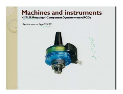
Now, this is a rotary dynamometer. This is another version of this KISTLER dynamometer and this is used for our drilling and milling experiments. It is 4 component dynamometer and it can may have 4 different computer F x, y, z and movement also F in x, F in y, F in z direction and also movement in z direction.
