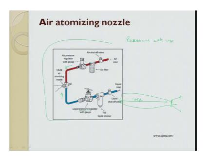
The next gadget I have in my hand is air atomizing nozzle. This is an air atomizing nozzle that also we call from US only. So, generally there are 2 types of setups for atomizing like for producing mist. So, this system that I am showing here is pressure setup. In this case, actually air pressure is there and obviously, liquid is there and liquid is also supplied through pressure.
