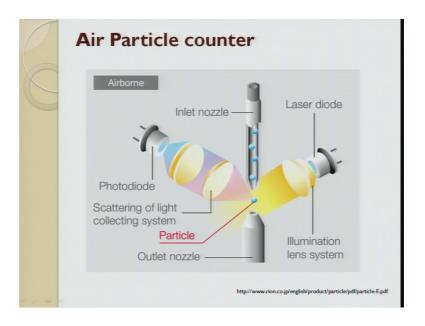
The principle on which this is working I will tell you. There is a light that is passing here, a photo diode is here, that is light is there scattered light is collected by the system and the particle, this scattered light produced a image here and this image is recorded on a diaphragm and that image is used to tell us the particle dia.
