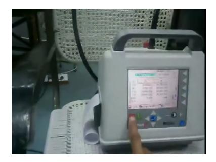
So, this is my air particle counter. That is collecting the mist particles or the aerosol those are generated; details about this we will discuss. This is one of the instrument that is been used here. Thus switch it off.
