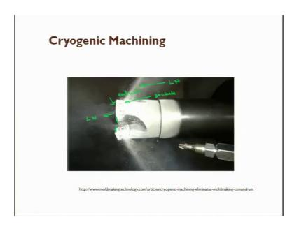
So, this is one of the figure here. This is my end mill and we have this jacket here from which liquid nitrogen is coming out. This is taken from a reference. And see it is also coming from this side. So, these are my cutting edges, this is the cutting edge here, this is the edge.
