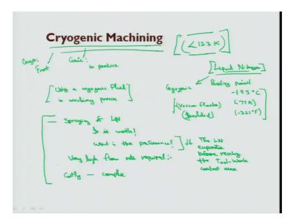
So, one other kind of the option or the green option there is cryogenic machining. What is cryogenic? Cryo means frost; this is cryo and genic means to produce. So, then cryogenic becomes the science that is associative generation of low temperatures then these temperatures are below 123 Kelvin that is the cryogenic. So, cryogenic machining is performing our machining process at this temperature that is cryogenic machining.
