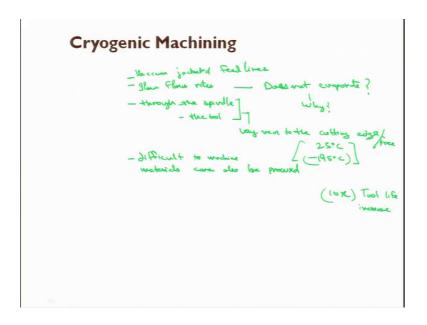
So, what is the new technology to overcome this drawback? So, new cryogenic machining technology utilizes vacuum jacketed feed lines that deliver the cryogenic fluid at slow flow rates. So how this slow flow rates could be effective, what happens? The fluid does not evaporate. Why? Now, what is there, this fluid is flown through the spindle only, through the spindle and through the tool and this is done very near to the cutting edge or maybe face.
