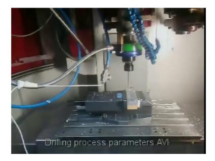
So, this is MQL-Minimum Quantity Lubrication drilling. So, you can see noise is coming here that is the kind of a peak noise. I have a nozzle here that is spraying with the fluid here. This nozzle from the white pipe the cutting fluid is coming and from the blue pipe on the top of the nozzle we have our air pressure. The pressurized air is coming up.
