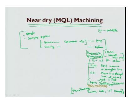
Now, next is near dry or minimum quantity machining. In this case, we already mentioned that 10 to 100 ml per hour of cutting fluid is sprayed. So, how do we do that? We need a nozzle here and we need a spraying system here. This spraying system maybe pressure spraying system or it may be using gravity only.
