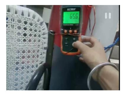
This is my sound meter that is recording the noise at each one second; that is, the second rate, the pulse rate; it is kept as one second. It is recording the noise and even the peak noise that you might have heard here, was also recorded here. So, this average noise during this machining and the peak noise these were be recorded.
