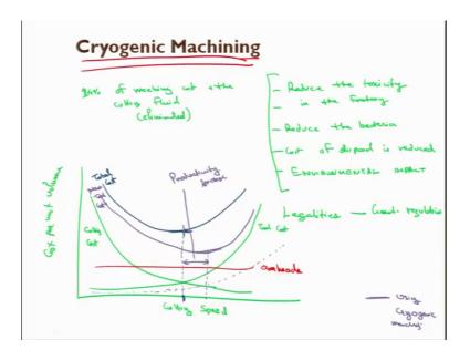
So, what was the motivation behind using cryogenic machining? We need to reduce the toxicity in the factory or maybe in the work environment, then similarly reduce the bacteria that are produced from the oily work environment or maybe from the cutting fluid, then cost of disposal that is reduced, then environmental impact the major thing this is also reduced.
