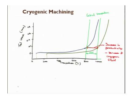
So, how does this tool cost low curve gets down, this I will try to elaborate here. So, when I plot my tool wear with temperature and if I say my machining is being coming out from 0 to 1000 degrees centigrade temperature and this is an absolute unit tool wear that is in mm and this is from 0 to 200, 400, 600, 800 and 1000 degree centigrade temperature is there and this varies from 0, 0.2, 0.4, 0.6 so on 0.8 mm.
