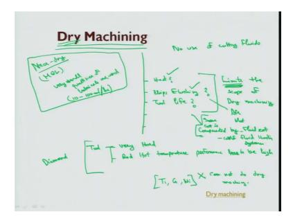
For this is the most radical approach is do not use the cutting fluid at all, a dry means dry machines that is no use of cutting fluids. Another process similar to this may be near dry, in near dry process that is also called as minimum quantity lubrication process in which very small quantities of, very small quantities of lubricants are used. This is near dry process. Now this small quantity may be from 10 to 100 milliliter per hour.
