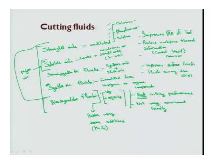
So, what are cutting fluids? Cutting fluids are used in metal machining for a variety of reasons such as cutting fluids improves life, improves life of tool then reduce work piece thermal deformation reduce work piece thermal deformation. That is it controls the heat
