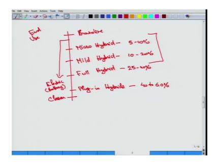
And the cars the concept is there even testing is done only thing is that mass production is not there micro hybrid cars what are this micro hybrid cars as this switch the gas engine off when the vehicle would normally be idling running the mechanical such as heater accelerator batteries etcetera efficiency grains are from 5 to 10 percentage in this case then we have mild hybrid cars.
