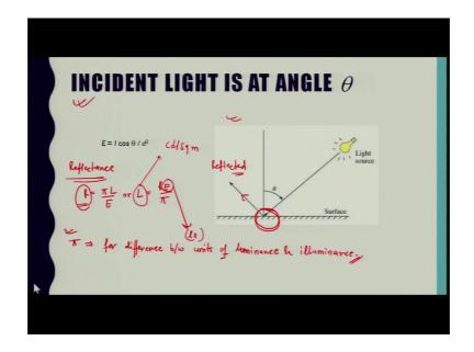
So, this particular incident light at some some sort of angle let us say theta. So, that we have described and now another aspect that we need to understand that when light shines on a surface some of the light is absorbed into the surface, where light is particularly incident and light is absorbed here and some of it is reflected from the surface.
