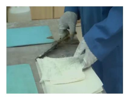
Now, next we are going to fabricate a simple composite using, we selective fiber, we will select a resin here and we will do fabrication. Now, this kind of fiber, we are selected, is chopped fiber and we will make a simple sheet of composite of dimensions 200 mm into 150 mm. Now, what we have here is, we have cut this, chopped fiber into pieces of the
