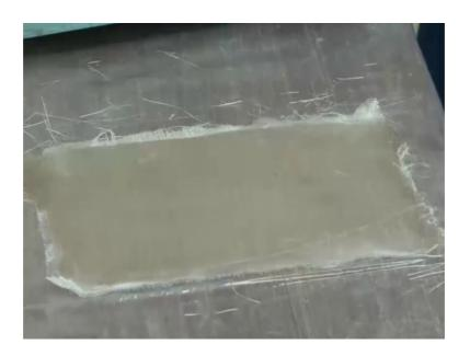
Now, we are ready with our final composite. So, in demonstration, we just had an look, over the types of fibers, we had used resin polyester resin, then we did fabrication of composites, this process which is used here is known as wet layer process or maybe hand layer process
