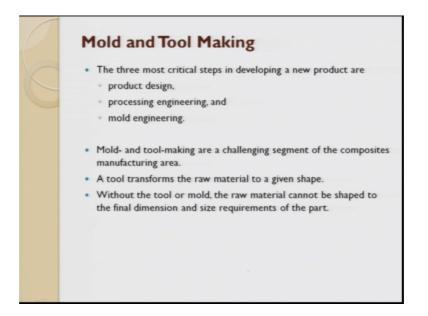
Mold and tool making three most critical steps which are involved in a new product development are product design processing engineering and mold engineering tool and die making or mould and tool making are a big challenge in the area of composite manufacturing. The tool transforms here raw material into a finished shape without a tool or a mold the raw material cannot be shaped to a final shape and the size required for the part.
