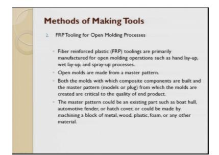
So, that are FRP tools for open molding processes, FRP itself is used as a tool. So, the pattern is made out of FRP, instead of making a wood pattern, instead of making a steel pattern we make a pattern out of composite itself and this is good enough for large area structural application parts, you want to do you can use fibre reinforced plastics as they are die itself.
