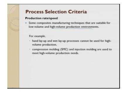
Some of the composite manufacturing techniques that are suitable for low volume and high volume production environment are for example, for low volume we will look for hand layup process, wet layup process, which cannot be thought of a high. High volume production in high volume production we always look for compression molding and injection molding where in which it tries to scatter to the high volume production requirements.
