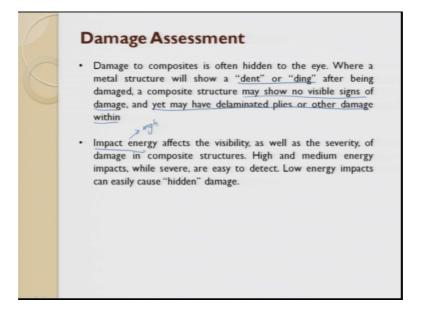
Any composite which undergoes a damage these are the repair procedures first inspect and find out where the damages come out with a strategy for repairing it, then try to repair the damage then after repairing please check for the quality assurance and then you go for finishing such that it can be put into good use.
