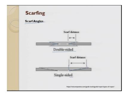
So, here is it. So, here you are damaged. So, here we prepare the double sided and then we put we find out the scarfing distance and then we try to put the layer. So, this is the scarfing angles. So, it can be single sided it can be double sided whichever you want you try to take and then you try to prepare. So, if you see that the scarfing and the distance is nothing, but from here to here we prepared such that you can have a proper repair patch.
