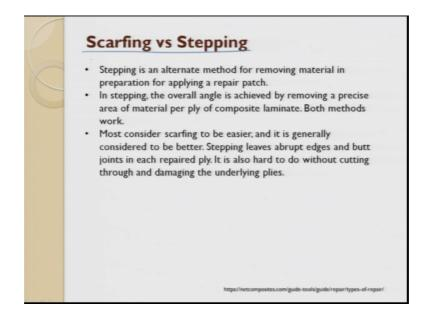
So, scarfing versus stepping; so, stepping is an alternative method. So, here in stepping; what do you do if we make it in to steps and in scarfing, we make it as a tapered angle. So, that is the difference. So, if you see the stepping is an alternative method of removing material in preparing for applying repair patch in stepping the overall angle is achieved by removing a precise area of the material ply of the composite laminate both methods scarfing and stepping works very good.
