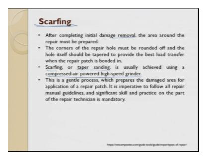
So, in this the strength is regained to a large extent. So, scarfing scaring after completing the initial damage removal the area around the repair must be ready. So, the corner of the repair hole must be rounded of and the hole itself should be tapered to provide the best load transfer when the repair patches is bonded to it.
