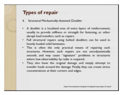
So, this one is called a semi structural plug or a patch which is done here it tries to take load then structural structurally mechanical fastened doublers. So, these are the doublers. So, here what do we do is we try to have bolt patch repair.
