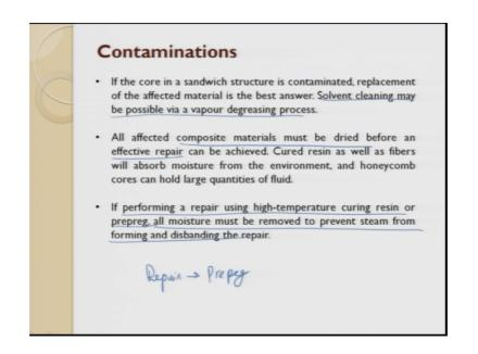
It is easy for a laminate suppose if it is there for a sandwich composite. So, in a sandwich composite if the core in a sandwich composite is contaminated replacement of the affected material is the best answer a core; suppose if the core; if it is not possible, then we have to look for alternatives. So, what we do is we do solvent cleaning and maybe possible, we will try to vaporize or we what we do is we try to degrease that part and then remove that part.
