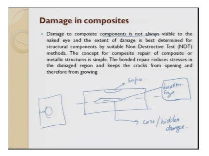
So, that it looks to be the same as the original part damage in composite component is not always visible by naked eyes. So, it can be on the surface the damage the if you take a composite the damage can be on the surface the damage can be on the core these damage are called as surface damage this damage are called as core damage or hidden damage core or hidden damage.
