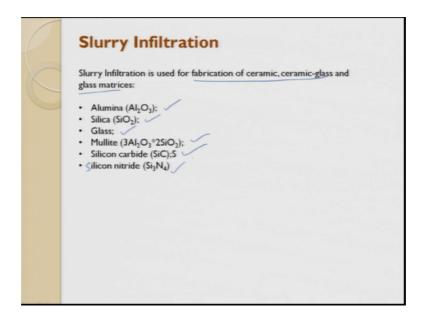
So, you get a clear composite ceramic matrix composite. So, this slurry infiltration can be the you can use these are the fabrics for fabrication of ceramic and ceramic glass and glass matrix alumina can be thought of silicon; siloca can be thought of glass mullite which is the form of a glass, then I SiC and then you can also have silicon nitride Si silicon nitride is also used in the in this slurry to; so that we can make the composites.
