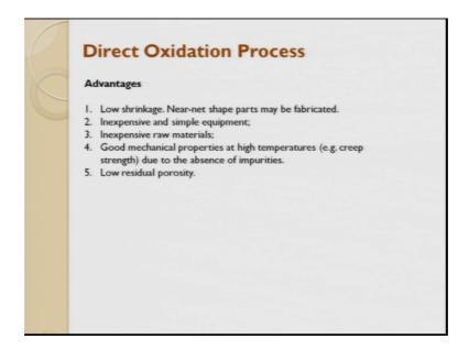
So, what are the advantage it has low shrinkage near net shape can be made, it is inexpensive because you do not need to have very high pressures and pushing and the raw material is also inexpensive, it has a good mechanical property at very high temperature in the presence and due to the absence of impurities.
