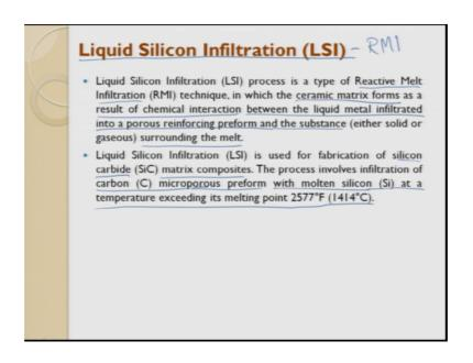
And the production cost is extremely high the next process of discussion is going to be liquid silicon infiltration process which is otherwise called as LSI liquid silicon infiltration process is a type of reactive melt infiltration RMI technique in which the ceramic matrix form as a result of a chemical interaction between the liquid metal infiltrate into a porous reinforced pre-form and the substance surrounding the melt.
