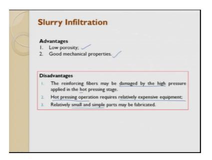
So, the slurry infiltration process it as an advantage of low porosity and it is has a good mechanical properties can be achieved because of this the disadvantages are the reinforcing fiber may be damaged because we are applying very high pressure and the 2 stages then the hot press generates relatively needs are relatively high cost equipment and they are used for making very simple and small parts using this process.
