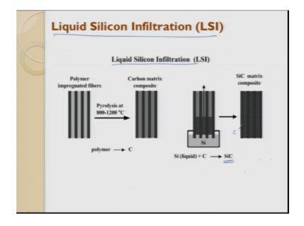
So, this is what it is. So, liquid silicon infiltration process polymer impregnated fiber I told you the common steps. So, that is there from there what happens it goes to pyrolysis it gets converted into a carbon. So, you form a carbon matrix composites right the next one is we try to put this carbon matrix composite inside liquid silicon and then through to capillary reaction this Si goes into this carbon matrix composite and forms SiC matrix.
