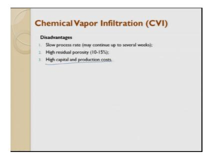
So, the disadvantages are this is a slow process the porosity even after all these things there is a porosity which is coming up 10 to 15 percent all the ceramic matrix composite fabrication process is highly capital intensive.
