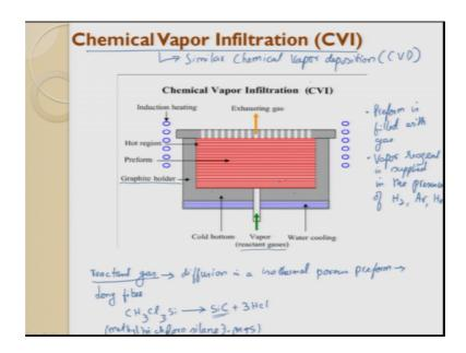
The next process of discussion is going to be chemical vapor deposition. So, in this process the ceramic matrix is composite is fabricated with reactant gas this gas what happens it undergoes a process of diffusion this diffusion in a ISO thermal porous reform.
