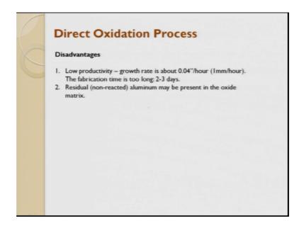
It is very good, it has very low residual and porosity in it the disadvantages are going to be it has low productivity and the residual aluminum may be present in the oxide which tries to react and form oxides and this will try to reduce.
