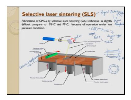
So, the other process which is called as selective laser sintering process this is part of rapid prototyping which is part of rapid prototyping technique. So, this is also used for
