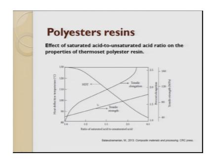
So, if you look at this graph it clearly says the effect of saturated acid to unsaturated acid ratio, on the properties of thermoset polyester resin.
