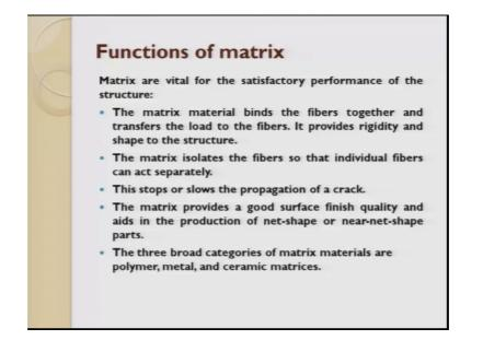
First thing is the matrix material binds the fiber together and makes were the load is uniformly transferred across the fiber.
