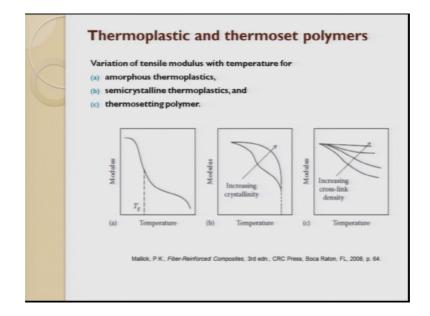
So, here are some of the various properties which we have compared. So, you can see here the first one is modulus with respect to temperature. So, here since it is a polymer it does not have a exact point of transition from solid to liquid, it gets into a zone and then it gets converted into a liquid form.
