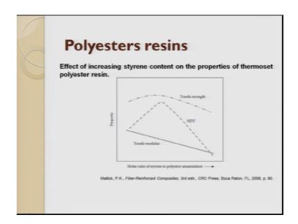
So, polyester resin the effect of increasing styrene content on the properties of the thermoset polyester resin, you can see that the molar ratio of styrene to polyester unsaturation. You can see what happens to the HDT curve and the tensile properties and tensile modulus.
