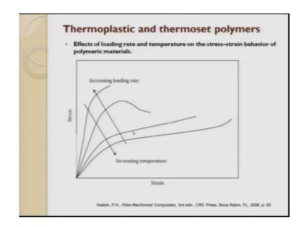
Because, this property tries to decide how the load gets distributed in the composite and what should be done. So, you take here this is stress this is strain. So, stress versus strain graph, so here let us take the influence of loading rate, if the loading rate pattern increases; that means, to say at higher loading rate the ductility falls down drastically.
