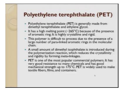
Next one is pet is polyethylene terephthalate is generally made out of dimethyl terephthalate and ethylene glycol. So, these 2 mix together to form PET as a melting point of 265 because of it is presence of aromatic ring, it is also highly crystalline and rigid in nature.
