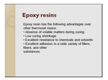
The epoxy resin has the advantage over all other thermoset resins these are the. So, it is the volatile matters during curing is one of the biggest thing, it has low curing shrinkage it has excellent resistances to chemical and solvent, it has excellent adhesion to wide variety of fillers fibers and substrate.
