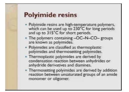
So, where the temperatures, where the polymer requires high service conditions; so we always go for polyamide resins or high temperature polymers, which can be used up to 230 degree Celsius for a longer period of time and it can also work up to 315 for a shorter period of time.
