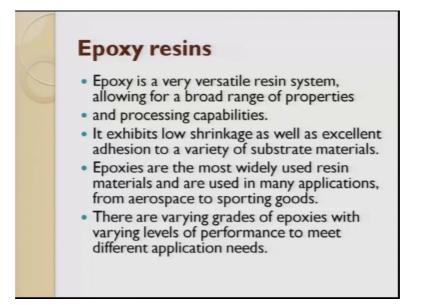
It exhibits very low shrinkage, low shrinkages very important because in a liquid form when you try to use a resin and when the resin gets cured; that means, to say when it is completely liquid is converted in to solid, the shrinkage if it is very less than the shape whatever you want you can easily get it done, if there is a shrinkage than this can be happening 3 dimensionally and it is little difficult to control the output.
