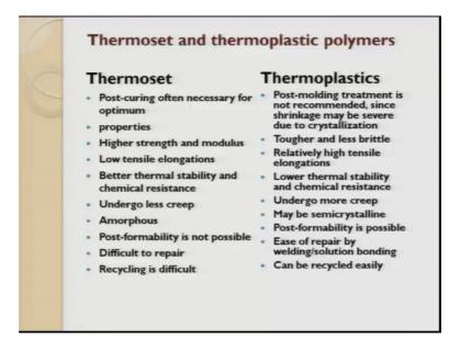
The post curing one thing you should understand the polymer, when you make a polymer matrix composite 100 percent setting never happens, the setting happens up to 95to 96 percent and over a period of time. All this cross linking are happened and small changes happen within the polymer and it becomes 100 percent cure after all longer period of time as for as thermoset is concerned.
