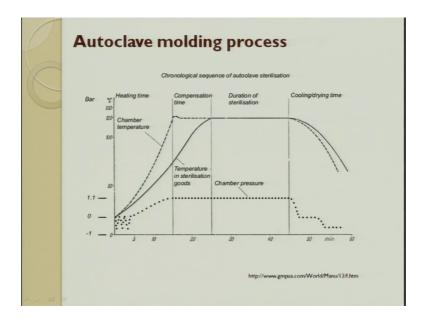
So, this is the chamber pressure. So, we always operate up to 1.1 and you can see the temperature going up. So, this is the chamber temperature which is preheat then you have a compensation time then you have a duration of sterilization and then you have a cooling period the temperature is a is the in the sterilization zone. So, this is what it is. So, the temperature initially goes high maintains it and then you try to get an output.
