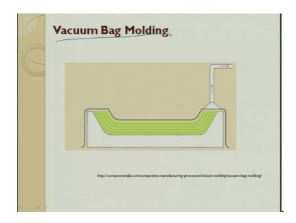
So, this is a schematic diagram of vacuum bag molding. So, we have several layers of reinforcement place and here is a vacuum which is there here is a bag which is there on the top.
