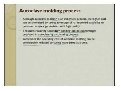
So, complex parts are only tried to get the output, the parts of the secondary bonding can be economically produced by autoclave by using co curing process. So, we will see what is co curing process little later sometimes the operating cost of the autoclave is also can be considerably reduced by curing many parts at a time; that means, to say one shot process you can do or try to have multiple parts in one autoclave process. So, by that we can try to compensate the produce.
