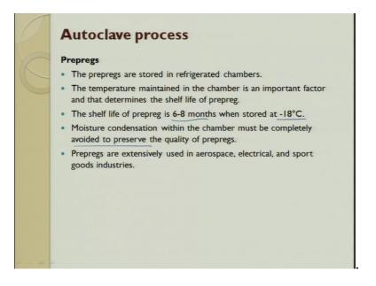
So, here the uniform fiber to resin ratio the variation will be as low as 2 percentage so; that means, to say you will get a very sound product. So, they are store in refrigerator because when you expose it to temperature it will cure. So, they are always maintaining at minus 18 degrees they have a shelf life of 6 to 8 months. The moisture consolidation within the chamber must be completely avoided to get a good quality output this is used for various applications.
