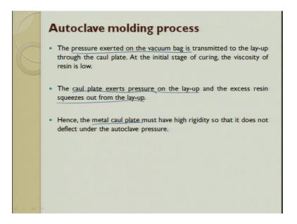
The pressure exerted by vacuum bag is transparent to the hand layer. So, that they can flow the caul plate exert pressure on the layup and the excess resin are squeeze out through the lay-up. So, hence we always use a metal caul plate must have very high rigidity to in the auto in the auto calve process. So, this is a typical cycle of an autoclave. So, you can see that the pressure which is maintained in bar the temperature is given this is the time in minutes.
