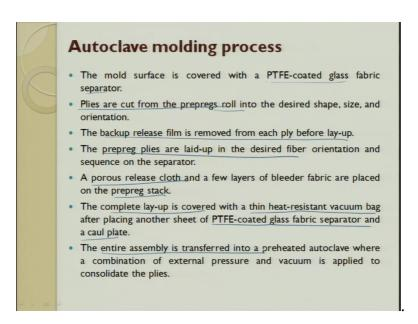
So, you put a you put the prepreg before the prepreg you try to put a small coating at the bottom releasing agent then what you put the prepreg then after that you put a peel ply
