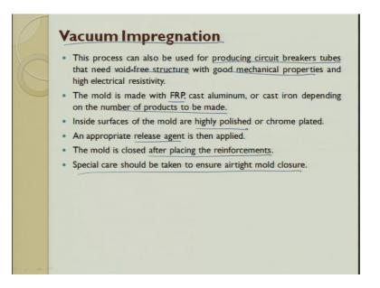
What is impregnation? The process which is used for these are examples I have given producing circuit breakers tubes that needs void free structures with good mechanical properties are always done by vacuum impregnation molding.
