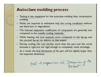
So, the tools here are very less in expensive. So, like a compare to a compression molding. So, here you make a small pattern or a mold or a. So, this can be made out of steel this can be made out of the pattern can be made out of steel, it can be made out of wood, it can be made out of a composite people have studied what is the influence of the basic pattern material over the output.
