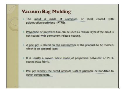
So, the mold is made out of the mode is a bottom surface which is made out of aluminum steel if it you want to have multiple process the polyester film can be used as a releasing agent the plies are placed on the top and the bottom of the product or the mold. So, the oven fabric of whatever it is you want to keep your placing it is quoted with glass fiber and the peel ply renders the curing laminated surface paint ability or bondable with the components.
