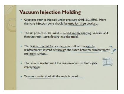
The catalyst resin is injected under a pressure of what is catalyst catalysis the catalyst is nothing, but to accelerate the reaction catalyst resin is injected at a pressure of 0.3 mega Pascals it is injected more than 1 injection point can also be used if you want to make a large component. You will have multi injection if you want to make a wind blade or if you want to make a closure for a complete car. You will have multiple injection points.
