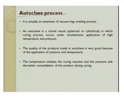
So, auto clave is another process which is used it is an extension of vacuum bag molding process.
