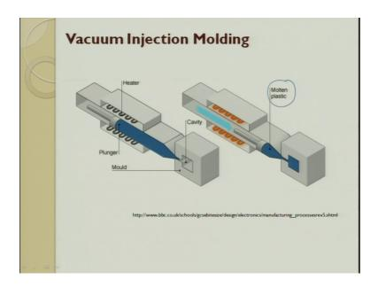
So, this is the heater vacuum injection molding this is a cavity you have a mold cavity you have a plunger through which the resin is heated in order to maintain the longer part life, What we do is we try to heat the resin and maintain it in the liquid state. So, viscosity is less. So hat it can be done. Here it is molten plastic is injected into the cavity. So, that you try to produce a part.
