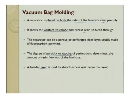
So, to go more the separation is based on both sides they it allows volatile material to escape the separation through the porous are perforated fiber layer usually is done by made out of fluro carbon polymers they have separators also applied the porosity can be reduce drastically there are bleeder layers where in which the excess resins are absorbed. So, it is like a cotton bleeder layer is like cotton where in which it observes the excess resins. So, that you get the sound product output.
