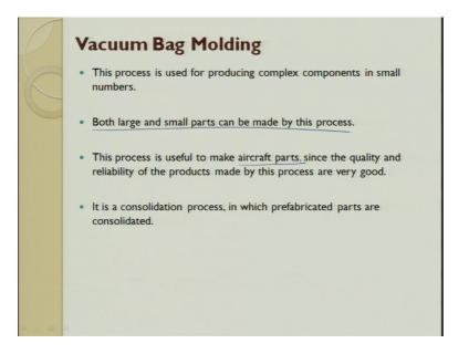
The vacuum bag holding this process is used for producing complex parts in smaller numbers both large and small parts can be made in this process for example, I told you aircraft parts windmill parts can be made and you get a you get a sound product the products that are fabricated by hand lay process can be consolidated by vacuum mold see what happens in hand lay process is?
