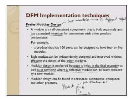
As part of design implementation technique design for ease of manufacturing is also there so, the last step is modularity. So, modularity means I make sub assemblies and these sub assemblies can get into n different outputs or customer products. So, a modular is a self contained component that is built separately. So, what happens means you have products these products will have several sub assemblies right this can be a, b, c and d you can have.
