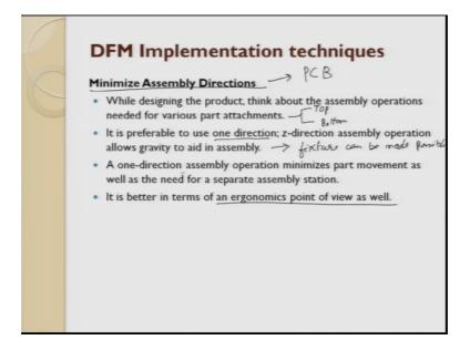
The directions the best example is PCB printed circuit board. While designing a product think about assembling operation needs from various part attachment I told you top and bottom which is top and bottom and also you can have sides and other things it is prefer to have only one direction why because the fixture can be made possible you can also see sir why not vertical.
