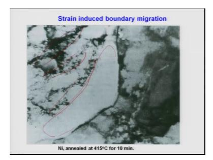
This picture is or nickel annealed at 415-degree Celsius temperature per 10 minutes after cold work, you can see the boundary which is there this boundary has moved from
