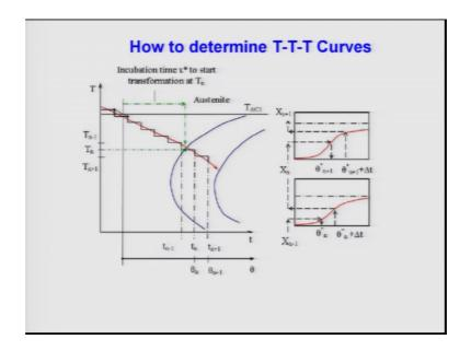
Passes time and you can actually see here at time theta n and at time theta n plus delta T we can actually determine the pass in a transformations differently. This is again a s curve here also s curve. So, one can determine different percentage of transformations, and then we can bring it there that is possible.
