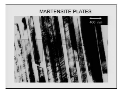
That is there on the plane between the austenite and the martensites, but mostly internal faults are more predominant in the microstructure. That is what I have shown you internal faults like twins very predominant in the martensitic plates.
