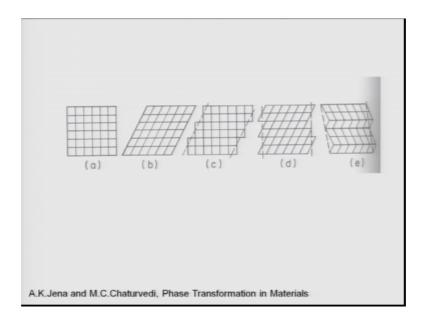
Suppose if I take a simple undistorted lattice as soon as a. And then started giving a shear strain, this is given a shear strain. So, one has bent one part of the crystal has become this bent with respect to the other. And again if you want to create invariant planes which will remain invariant in with respect to the matrix, then what is require is to give a slight distortion like that you see this is a slight plastic distortion given. So, at any place do get move.
