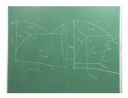
So, let me just do it on the board. So, as we have seen in the phase diagram looks like this. This is 660 degree Celsius, because this aluminium alloy temperature, and this is weight percent copper and we are not drawing it.
