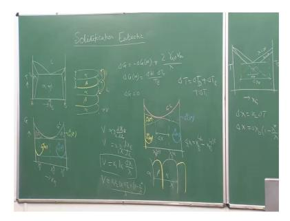
So, as I told you, let us first draw a phase diagram which shows the eutectic growth. As usual it is a phase diagram with two terminal solid solutions liquid transform to two phases alpha and beta, at the eutectic temperature, and we are going to discuss only the case for which the composition of the alloy is exactly same as eutectic; that is equal to X E ok.
