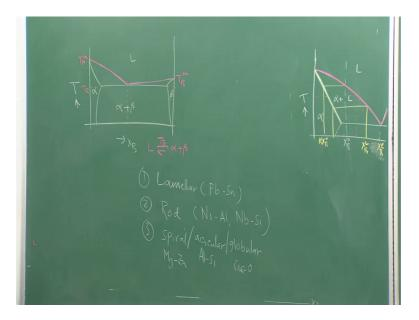
You will find many phase diagrams where eutectic is widely present the simplest eutectic phase diagram with 2 terminal solid solutions it is like that. So, alpha beta the 2 terminal solid solutions and eutectic is basically the lowest melting solid in this phase diagram as you see here both the liquidus is going down. And they are meeting at a point whose temperature is lower than the melting temperature of pure A and melting temperature of pure B.
