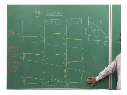
So, we have been discussing about solidification of the alloys x p 0. And I told you that the most realistic situation of solid profile is this one, the last one or the bottom one in this in these pictures. So, let us assume that we have a solid build up and the in this at the interface.
