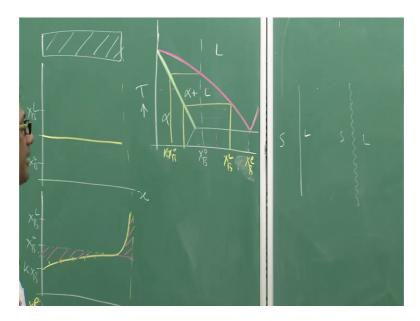
This fluctuations can lead to interface perturbed interface will become perturbed; that means, I can develop some sinusoidal perturbations on this surface, you see this is a sinusoidal curve you can also have co sinusoidal or any other such kind of perturbations now the question is this fine because of compositional change or temperature grad temperature variation according to interface certain kind of perturbation has developed acceptable understandable.
