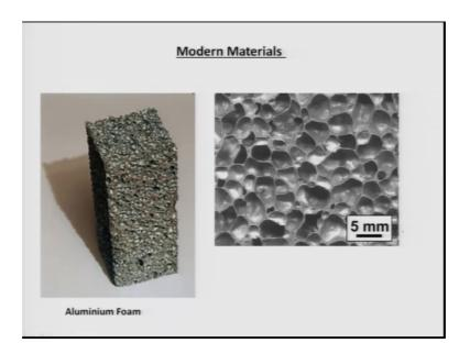
Now, it is people actually all talking about metallic foams, foams actually were important industrially because foams are used in the as a soft cabs absorber in the cars or even the you know different applications, where you need a ballistic things to protect it protect ballistic armor basically to protect from the bullet us. So, foams actually also made from liquid basically the foams are made.
