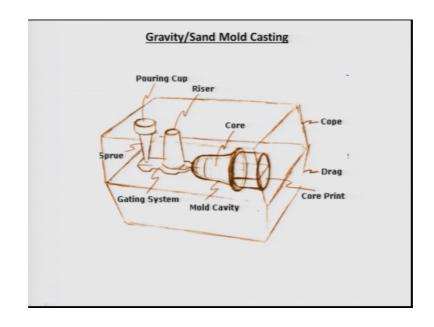
So, after the casting is made these 2 pieces are cut off by using some acetylene flame and the casting is separated.
