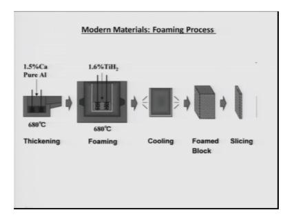
This is aluminum as a foam, you can actually have aluminum melt with little bit of calcium and then calcium actually stabilizes the foam basically foam is nothing but when
