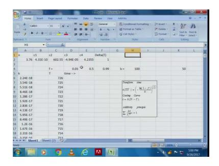
Have a lot of data I gave already input this is for a particular plain carbon steel here we are looking at austenite to pearlite transformation and what I have here is in this column I have temperatures starting from just below the eutectoid transformation temperature and then going down to over a entire large range of temperature out here is the value of k which varies as a function of this temperature.
