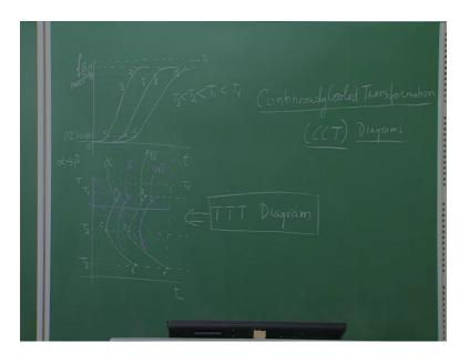
So, I have my fraction transformed beta phase, this is my time axis and let us say at some particular temperature this is fraction 1 this 0 and let us say this particular transformation kinetics given by this curve is at a temperature of T 1 where T 1 is less than the transformation temperature T r.
