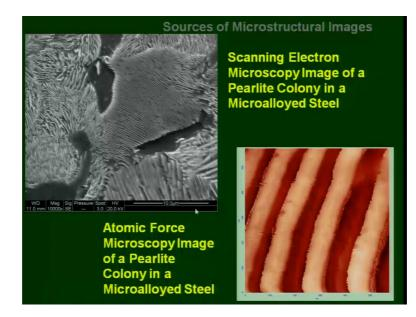
We can this is an image of a few pearlite colonies in a in a steel. Here we may be interested in measuring the inter leveling spacing again stereology can help us in doing that. This is just a magnified image of the same thing in a atomic force microscope.
