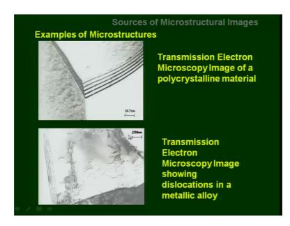
Now, these are projected images in a transmission electron microscope of polycrystalline material. This image shows 3 boundaries meeting at a triple edge, while the image at the bottom here shows this location and stereology can be used to determine for example, the density of dislocation which is line length per unit volumn.
