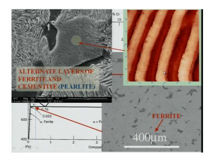
This is what kind of microstructure one would see. That you have a matrix which is essentially ferrite and there are re darkish regions as you can see, which if I zoom into one of these regions and looked at the structure under a scanning electron microscope then this is what I am going to see.
