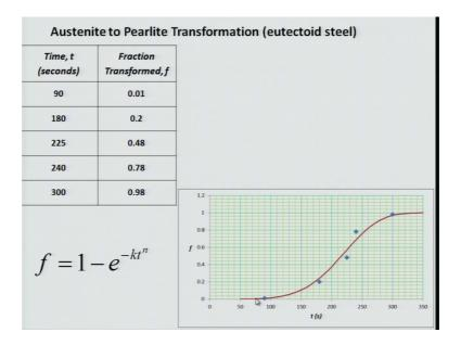
So suppose and this is an experiment in which some data has been collected of austenite to pearlite transformation in a eutectoid steel. So, and this temperature here though it is not mentioned, the temperature of the salt bath was kept at 660 degrees centigrade.
