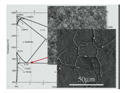
One can see that there is a network of phase precipitated this is the cementite phase, the proeutectoid cementite that forms and this cementite does essentially heterogeneously nucleated at the grain boundaries. When the temperature reaches below the eutectoid temperature than the remaining austenite transforms to pearlites. So, all of this regions within that is all pearlite.
