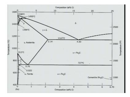
So, the and if one looks at the iron carbon diagram this is the iron carbon diagram. Here you can see that you have this is the usual iron carbon diagram which you already know.
