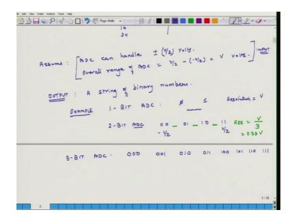
So, the overall range of ADC is what? V over 2, minus v over 2 that is v volts; so, it can handle at the max plus v over 2 and at the min v over 2 volts. So, it will overall range v volts.
