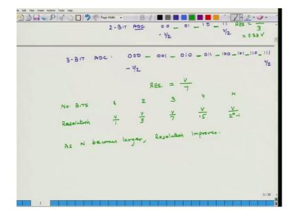
And how many gaps are there? 1, 2, 3, 4, 5, 6, 7, so our resolution is equal to what? V divided by 7, this is a pattern here. So, number of bits let say 1 bit, 2 bit, 3 bit, 4 bit and resolution is what? V over 1, v over 3, v over 7; in case of 4 it will be if you do the math and do all this type of analysis you will find the that is v over 15. So, I can make a
