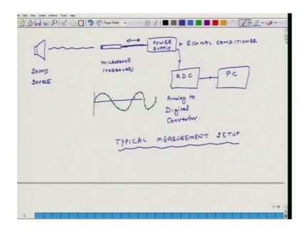
So, we will start with measuring sound. So, let say there is a sound source. Now, here I am making a schematic for a speaker, but it could be anything. So, this is sound source and it when it sound and let say we want to record this sound source so that once we record the sound signal, we can analyze it in detail understand it and take whatever actions we want to do.
