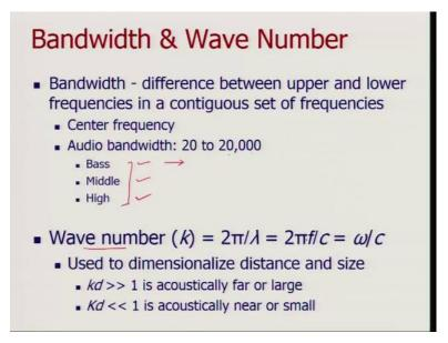
The next thing I would like to talk about is a bandwidth. So, we have already discussed, what is the bandwidth? It is a bunch of frequencies lying between an upper limit and the lower limit. So, that is what it and each bandwidth has a upper limit and lower limit and a central frequencies, the overall audible bandwidth for human voice or human hearing is 22 to 20000 hertz. So, that is equal to 3 decades because the ratio of 2000 and 20 is 310 to the power of 3. So, that corresponds to 3 decades.
