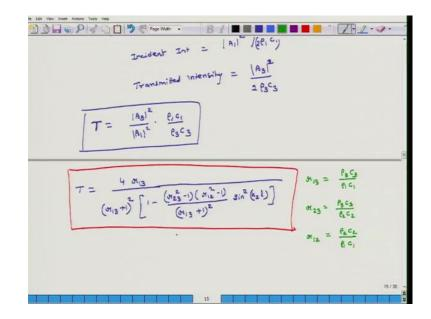
So, T equals A 3 square divided by A 1 square times rho 1, C 1 divided by rho 3, C 3. So, this is what we are interested in is how much energy we are putting into the system and how much energy is getting out of the system. So how do we calculate it from these four equations, first we calculate A 3 over A 1 and then we find out the magnitude of A 3 over A 1, square it and multiply it by rho 1 C 1 divided by rho 3, C 3 and we will get the answer, but still you know is that particular ratio.
