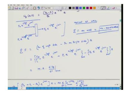
Let us look at couple of other factors. So, we want to know that when the sound is striking the wall as a shown in this picture, the wall is going to vibrate. So, what is going to be the velocity of that vibration?
