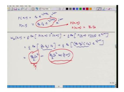
So now, let us look at the relation. For power we had defined power per unit area is equal to what. So, we are going to evaluate at x is equal to 0, so I will put that thing here. So, that is equal to half of real of P complex pressure amplitude times velocity its conjugate 0 omega plus half of real of P 0 omega U 0 omega e 2 j omega t.
