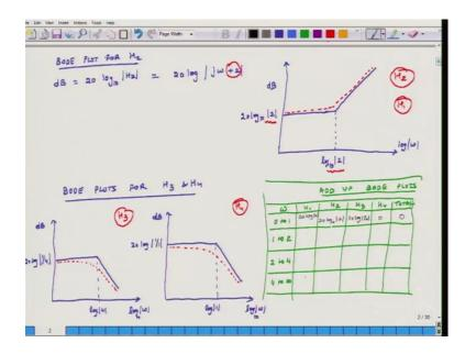
This is for H 1 and H 2 and next we will develop Bode plots for H 3 and H 4. So, we are going to directly develop the Bode plots because I thing we have done sufficient amount of practice. So, both of H 3 and H 4 are simple holes they are simple poles. So, what; that means, is that their Bode plots. So, my horizontal axis in both these cases log of omega and on the vertical axis or y axis I have decibels.
