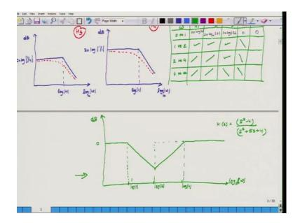
What we will do is we will now construct the overall Bode plot. So, overall Bode plot vertical x is in decibels. So, first we will do is we will marked down different points. So, first is 0 to 1. So, this is log of 1 then 1 to 2. So, this is log of 2 then 1 to 4 2 to 4. So, this is log of 4 and then 4 to infinity.
