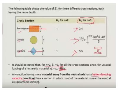
Let us see that type of a case so here we have considered 3 cross sections one is a rectangular cross section another is a circular one and the third one is a diamond cross section so rectangular circular and diamond cross section and their thickness is the same in all the 3 cases now the beta C for N equals to 2 is actually also same if you try to evaluate we will see beta C for N equals to 2 is not changing but Beta C will change for N greater than 2 like for N equals to 3.
