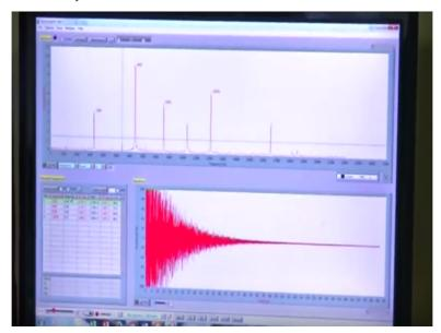
Now if we go to that then we will see that the frequency has actually reduced it is 3289 harge and also the amplitude in comparison to 23.7 now the amplitude is 4.29 so the amplitude has actually come down. One-fifth of the amplitude that it had when there was no such holes and the viscoelastic inserts that was there in the system so that is a fantastic improvement that we can see.
