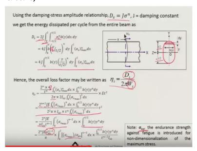
Now we also know that the damping stress amplitude relationship which I said in the very beginning that is what we are heading to is that a Loss Factor definition so in which we need the damping the energy that is dissipated which is J Sigma to the power n so the energy that is dissipated per cycle is J Sigma to the power n by 2 pi and the ratio of Plodder loss factor is this divided by w s.
