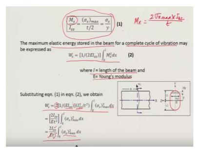
So that is the simple theory of bending so with this kind of conditions if we next actually look into it that our relationship the first equation is MX over izz as Sigma X max over T / 2 which is equals to Sigma X over Y that is what is our first equation.
