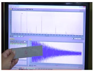
We are now going to show the frequency response function first for this solid aluminium bar and as you can see. Here that there are several frequencies that is appearing as we hit this system and we have chosen this frequency the second frequency which is 3366 harge and its amplitude is 23.7 and the quality factor is 7.79 into 10 to the power - 4.
