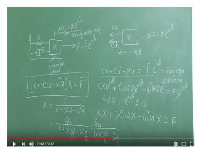
To do that let us first draw a single degree of freedom system. So let us say this is our boundary and we have a single degree of freedom system which has a kelvin Voight model type of a damping and the spring and the damper is attached to a mass in this case and the mass is resting on frictionless wheel. So these wheels are frictionless.
