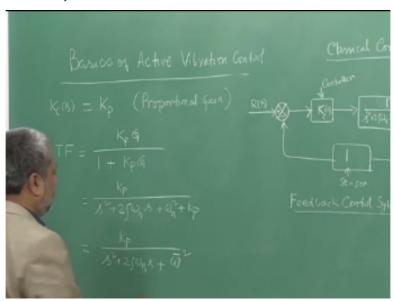
So in this case we will make 2 assumptions one is that this Hs will consider it to be unity, that means the sensor will have 2 dynamics, it will be proportionately feedback the output and compare to the Rs and then the whole system will run. So that is one thing and secondly this is tabulated in such a manner that this simply became unity for us calibrated in such a manner and that is what let us say is the very simplified system for us.
