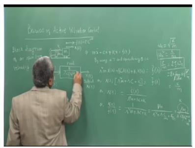
So we are going to talk about basics of active vibration control. To discuss this let us consider a simple block diagram of a vibrating system as a plant. So first we will take up block diagram of an open loop vibrating system. Let us see how we can translate the kind of the graphical representation of a open loop system in terms of a block diagram. So we have a mass M, K is the stiffness.
