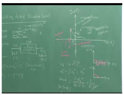
So let us try to clock these roots of the second order system and see what does it mean for us in terms of vibration control. So if clock this 2 roots what I am going to see is that we can start with an assumption that in a generalized case there is a real part and there is an imaginary part of these 2 roots. Now there are several possibilities of the roots. First of all can these roots being this side no if we consider then it will be an unstable system.
