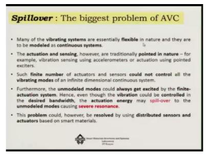
Well active vibration control has certain basic problems for example it adds energy to the you know vibrating systems, so it may also create instability because it is adding energy to the system. Consider that you have the active vibration system which is adding you know which is working on a vibrating system which is having a motion like this and it is suppose to so that means at this moment the structure is going up.
