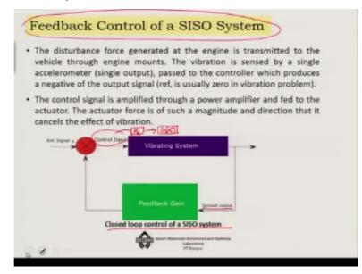
So first we are going to concentrate on the feedback control of a SISO system for vibration control. So here is this control structure again you have the vibrating system, you have a control input here, so that means the controller is actually integrated here, so if you remember that you have this Kc there and there is this plant gs all of them let us say that they are integrated in this vibrating system.
