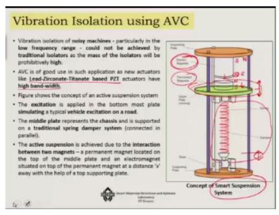
There is another popular one it is based on the control of the magnetic levitation and that is for example in this particular cases you can see that there is a spring here and the spring was damper system, is a traditional system and this is a place here and the plate has a permanent magnet in it, okay. So the whole system is resting on this spring damper system and it is a single degree of freedom system, which has a permanent magnet in the top.
