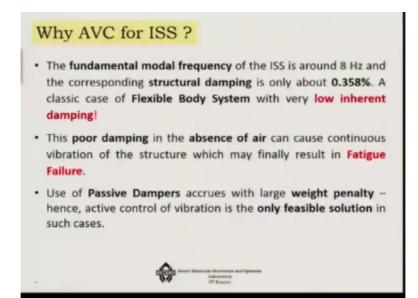
The fundamental modal frequency of this international space structure is about 8 hz and its structure damping is phenomenally low, only 0.358%. So this is the classic case where you have a flexible body 8 Hz you know fundamental frequency is very flexible and once the vibration starts it will not stop because the structural damping is very low. It has a very low inherent damping.
