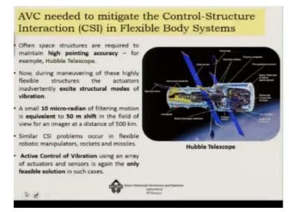
There are also some classical problems which we call as control structure interaction or CSI and that is particularly useful for any flexible body not necessarily for international space station. So one of the examples is where for example you need a very high pointing accuracy like in Hubble Telescope. Durgin maneuvering of Hubble Telescope you now if you excite in an inadvertently the structural modes of vibration.
