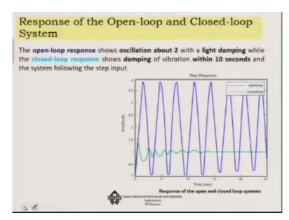
So with this system if I apply this particular controller then what is going to happen, you will see that in the open loop such is the amplitude huge amplitude, whereas the step signal that it has to it is suppose to follow in the close loop system once I close it you can see that within about you know oscillation of about 2 cycles itself within something like a 10 seconds, somewhere like this.
