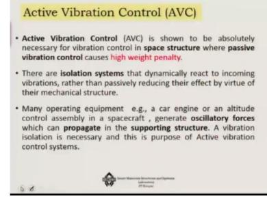
Now this was initially very much important for space structure where the traditional passive vibration control strategy was not welcome because there was a high weight penalty in such a system. So this kind of isolation systems that can dynamically react to incoming vibrations rather than passively reducing their effect was actually you now was a very welcome idea.
