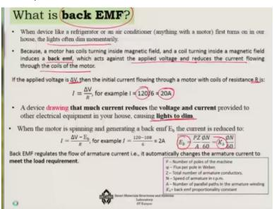
Will find that one important thing that will come into the motor model is called the back EMF ok, in motor actually you need two things one is called the armatia constant which will be knowing it typically depends on these you know coils, the coil density, coil materials etc., but the back EMF also is an important factor and you might have noticed it many times in your day today experience, suppose whenever a refrigerator or the air conditioner.
