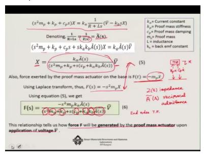
So, if you look at it, that if I combine the two equations and going to get this particular relationship and a little bit advanced if, I put one over R + Ls, now the R+Ls this LS in R+Ls can be written as the impedance. So Zs is actually Zs is actually the impedance of the system and A tilda is actually reciprocal of the impedance. So this is the reciprocal and it is also known as admittance.
