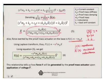
As you can see in this case, that this kpx + cpx dot the total of them is equivalent to what is the called the mpx double dot part of the system. So, the force that has to generated, has to be the negative of it, because it is in the opposite direction. So, then Ft is –mpx double dot, now if you use laplace transformation then it will become –s square mpX and now you can combine this 2 equations together.
