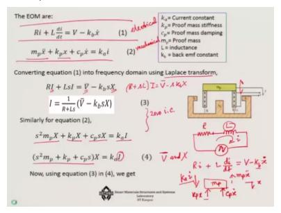
So, if we look in to the governing equation of the system, so, what we have is that we have two systems with us, one is an electrical part, so, let us first discuss the electrical part in the electrical part as we have seen that we have a you know resistance or and along with that in a series we have an inductant scale and we have a voltage source here from the motor okay and there is a direction of the current which is flowing through it right.
