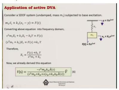
Ok, so, now we will be now talking about how we can apply this proof mass actuator in assistant which is undamped or under damped. Now let us say we disregard the damping part of that system, and let us say that the mass of the system for whose vibration I want to control using proof mass actuator is M1 stiffness is K1 and it is subjected to a dynamic force which is coming the source is the proof mass actuator.
