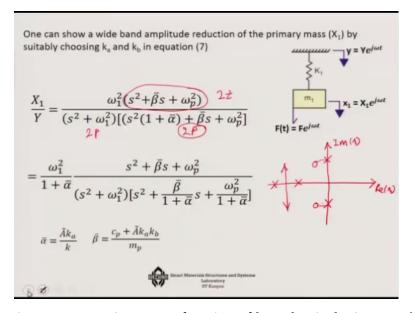
So, what we are going to get now is X1 as a function of k1Y that is the input and the voltage that have applying to the system. So I have a mechanical excitation this is the mechanical excitation part, it is just a post with two things right and this is the electrical excitation part. And, I am trying to surprise the mechanical excitation with the application of the electrical excitation. Now when A tilled s let us say the a very special case where you know the admittance is constant.
