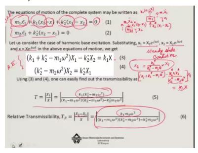
Let us now consider that what will happen if the x is x e rest to the power j omega t, let try to imagine and then x1 is the displacement of m1 let say this is also harmonic and that is x1 e rest to the power j omega t and at the same frequency an x2 as x e rest to the power j omega t. Now this will not happen immediately to give our basic citation, this **is** will happen when system will under steady state condition.
