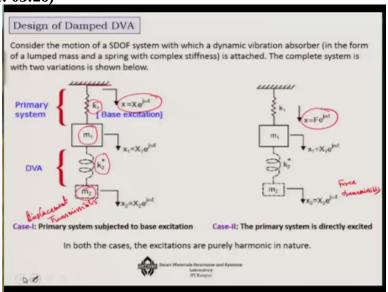
So here we have the primary system as has been shown in here K1 is the stiffness instead of Kp here we are denoting as k1, m1 is the mass and then k2\* is the actually is the complex stiffness and m2 is the is the mass of these secondary system. Now such a system is useful for 2 different
