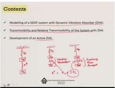
So we will talk about that how to model a single degree of freedom system with dynamic vibration absorber and then will talk about the transmissibility and relative transmissibility of such system and finally also will talk about an active dynamic vibration absorber. So just to keep yourself you know intact with the subject if you remember a warier said that suppose you have a simple spring and a mass system.
