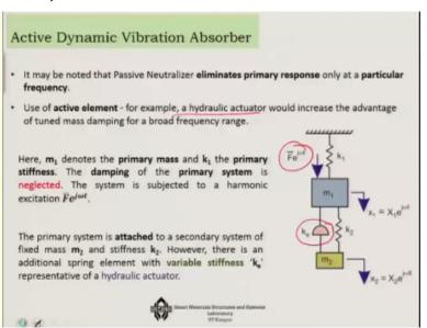
Now from here we need go to the case which is known as active dynamic vibration absorber, so, in the passive case, at least the dynamic vibration absorber case the most generalised case is better, because you have additional point with you pointer with you, which is the damping part,
