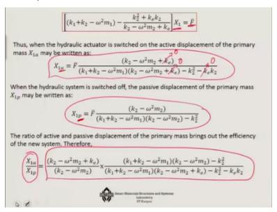
With that now we will be able to find out that what is x1 that is the response of the primary, and subjected to a force amplitude F bar, so, this is what the expression that will come out you can try using these last 2 steady state equation and this what is x1 a and if I put these K to the 0 this k 0 this k 0 then I get a simplified form where that active part is not that, the hydraulic control is not there.
