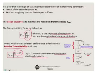
Let us say that we are taking the first case where we are having a transmissibility as X1 over X. Where x1 is the amplitude of vibration of m1, and X is the amplitude of vibration of the base, so, this the base excitation problem, ok, and x1 is you may also think of this way that X is the input to the system, and is the output response of system, so, this is something like an output over input.
