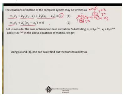
Now what will be the equations of motion of these systems. So in this case it is only subjected to base excitation. so that means if we try to draw this part if you remember what are the forces we are getting subjected to so m1 was undergoing a so there is a these direction of movement of m1 x1 so that means there will be an inertia force m1 x1double dot that is what is our faster here and then you also have in this case the spring k1 which is actually you know there is a base excitation there.
