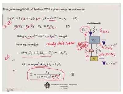
So, as you can see here that under such a condition now the right hand side is not 0, so, we have m1x1 double dot, which is the inertia force here, if you remember, that this is what we have and k1 x1 is also for here, that's the spring resistance k1 x1 and then k2 this part k2 x1-x2 that is the resistance that is coming from the bottoms that is this part and then we have the force excitation which is a bar e rest to the j omega t, in the right hand side here.
