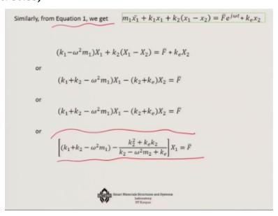
Now in this case then we can get the first equation of motion work on it and this will be final form of the first equation of motion so it this is the steady state form of the first equation on
