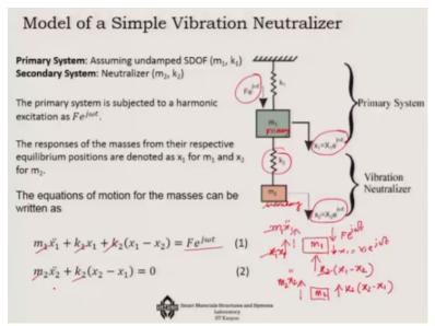
Now let us look into the model of a simple vibration neutralizer or tune mass damper. Stock bridge damper is one such example, so here you have a primary system, so this is the primary one and this primary system is getting excited by harmonic excitation and let say the excitation response is also harmonic x1 which is capital X1 as the amplitude times e rest to the power j omega t and the secondary system we have added a stiffener.
