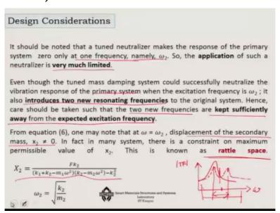
Now what are the design considerations for it, it should be noted that a tune neutralizer makes the response of the primary system zero only at one frequency that is at omega2, so the application of such a neutralizer is very much limited. There are some cases which will see where we can change this but in this case definitely it is very much limited and a even though
