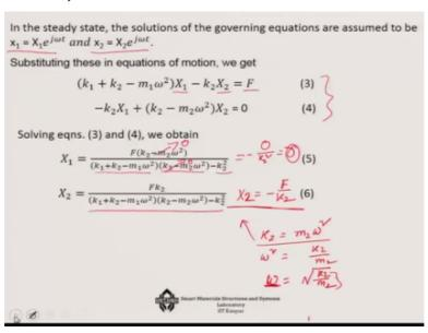
Now in the steady state, let us X1 as X1 e rest the power j omega t and x2 as capital X2 to the e rest to the power j omega t, because, we are only looking for the steady state solution. If you do so, then e rest to the power J omega t will cancelled from both the sides. And we will get these 2 algebraic expressions it which you will have X1 X2 and F. So, X1 X2 will be the 2 unknowns and there are 2 equations we should able to find them out.
