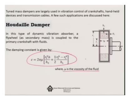
Is the Houdaille damper and in this of course there is damping constant that is involved in it, because these part in a Houdaille damper is filled up by viscoelastic fluid. So, if mew is the viscosity of the fluid, then we get this type of a damping constant for the system. Of course strictly speaking this is a case of what you can say is a case of auxiliary damper because it is damping that is coming in to the picture.
