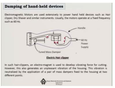
In here it another case we have the damping of hand held devices like say for example electric hair clipper, in this case the excitation is coming mainly because of the power supply which is above 60Hz, so, as this excitation is happening you can add a tune mass damper you can actually see that almost all such hair clippers will be coming up with the some more other form of the tuned mass damper.
