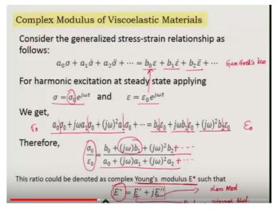
Such a change well we have the generalized stress-strain relationship which I earlier said as generalized Hooke's law we have that with us that model if you remember which we have used for obtaining the material parameter so in that model if I write it in long hand then it is a 0 Sigma a 1 Sigma dot a2 Sigma double dot etc that equals to B 0epsilon B 1 epsilon dot B 2 epsilon double dot etc now you imagine that I am giving either a forced harmonic excitation.
