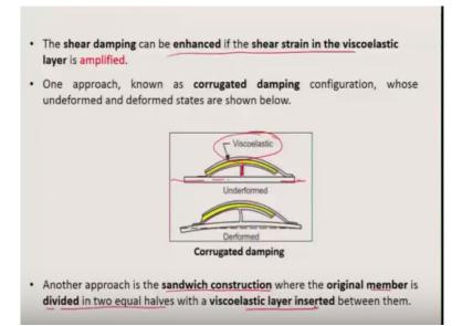
So this parameter G itself so this is how this whole thing behaves in terms of a constraint layer system depth now you can also make because the sheer damping is actually much higher than the flexural damping so you can try to enhance these shear strain by actually artificially constructing a system in which you keep this entire viscoelastic layer and the constraint layer away from the neutral axis of the system by developing you know a kind of a extension corrugated kind of a configuration.
