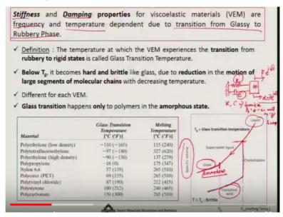
Now stiffness and damping in comparison to all other materials for viscoelastic materials both stiffness as well as damping they are actually frequency and temperature dependent. So which means, that when you are applying a dynamic load and if you remember that you know single degree of freedom system. Right. So if I just draw that single degree of freedom system for your reference this was the Kelvin Voigt model of the viscoelastic material.
