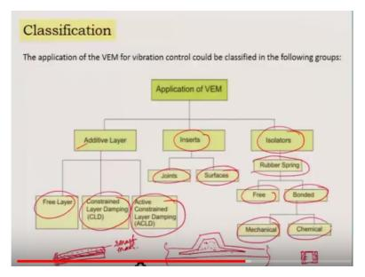
Now let us see that what are the applications of this viscoelastic material for particularly keeping vibration control in mind well there are huge applications I have sub divided them into 3 parts additive layer where viscoelastic material is applied as an additional layer so let us say this is what is my structure which is vibrating and I am applying a small layer of viscoelastic material so this is an additive layer and this additive layer.
