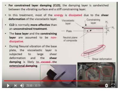
So we have to judiciously choose the modulus of elasticity ratio of the system now constrained layer damping is little bit different from the free layer damping as you can see
