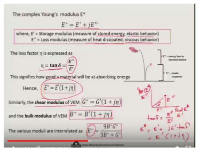
We call it as the loss modulus so these are the 2 parts that are there in the complex expression of the modulus of elasticity now we can also find our old friend Loss Factor now with this definition because e star is e prime + j e double prime e star Y prime I told you is the storage modulus which is the measure of the stored energy and it depicts the elastic behavior.
