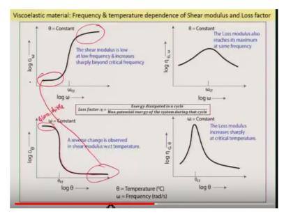
If we first look into it with respect to temperature that at the low temperature in this is your glassy phase and here it is brittle yet it is having a high modulus of elasticity but as the temperature increases this motion increases and there is a sharp fall in terms of the shear modulus now frequency behaves just the other way around that means whatever is good or whatever happens in a low temperature you will see that is going to happen at a high frequency level.
