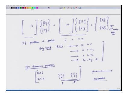
So, this is the global assembly, the assembly of all the equations then I get a big m matrix which you have four sub matrices and then I have a; so when I am trying to solve this, if problem is static which means u double prime, v u double dot and v double dot are 0, then I do not have to worry about these terms. In that case, I only need what, I only
