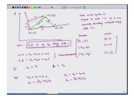
So, this is my global coordinate system x y and this is my triangle. So, we have side one side 2 and we have side 3 we have node one node 2 node 3 the global coordinates of this are x1, y1, x2, y2 and x3, y3, x1, y1, x2, y2, x3, y3 they are the global coordinates.
