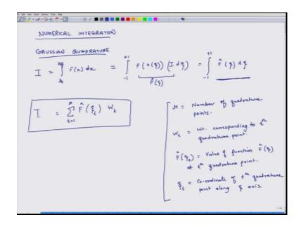
So, as said we will continue discussing numerical integration for starters. And if you remember we had said that for Gaussian quadrature, if I have to compute an integral I within the limits x B to x B and I have to integrate a function F x d x. Then the first thing is that I transform this integral into natural coordinate system. So, my limits become minus 1 to plus 1 then F is a still the same function, but x gets replaced by a function of zeta and then d x gets replaced by J times d zeta.
