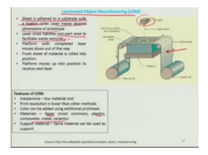
The other technology which is widely used is again is the animated objective method manufacturing, where there is laminar sheet which is made up of some kind of paper and plastic or composite or metal ceramics and what basically this technology does is that. In this case you know the sheet is near to the substrate with the heated roller and there is the laser which traces the desired dimension prototype and cut it off.
