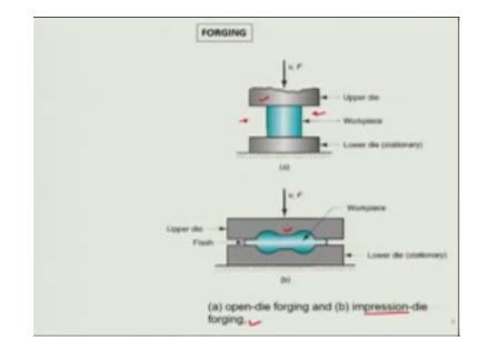
Like forging where either can have a open type forging case and there is a very nice illustration in the notes as well where we talk about how frictional force related to the die here and the expanding metal would vary there would really a point where the deformation would be at the same velocity as the or the force of the formation of the stress total principle stress would be the same value as the frictional force occur between the dies and the work piece.
