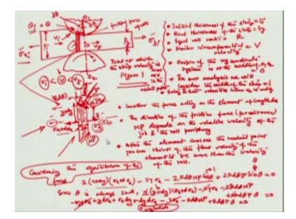
So if you look at basically this earlier figure right here you know that this is the direction of the roll pressure P and it is a triangle  $\theta$  with respect to the horizontal so we are talking about this separating roll force which is a component of this p which actually is imparted by the sheet on the roll, so that roll try to separate out because of the rolling process.
