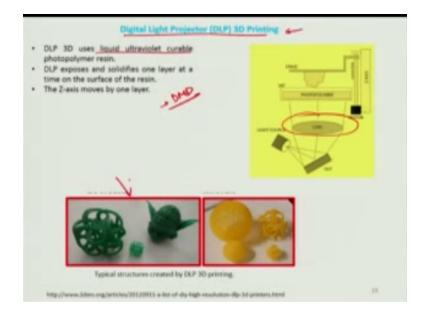
So then there is digital light projector based 3D printing, which I had already illustrated earlier that instead of a you know of single laser points standing the whole structure in this particular case it is basically a digital light projector which is also keno as DMD digital micro device, which is actually used by scanning and rotating a ray of very small mirror, so that the limits can be formulated and the idea there package which can section, a particular geometry.
