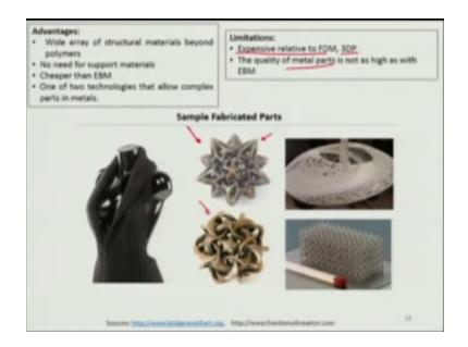
There are some part here manufactured by simple SLS process, obviously it is expensive related to the few position modeling or even the 3d printing done earlier by the other step but also there is other limitation the quality of the material bars that could produce nearly as not as high as a machine would produce and in this case you may not serve the distance requirement that is need by some of the dynamics machining to produce such parts.
