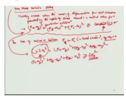
So this is the ultimate state of the distortion energy case you know this transient strain energy case so when we are talking about the coordinate frame which is really parallel to the directional of direction of all the principle stresses so having said that now the if we apply really this criteria
