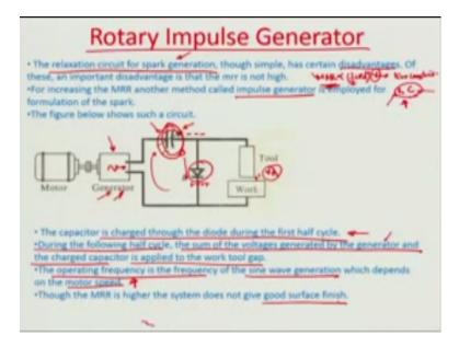
And this is typically having some advantages over the relaxation circuit for spark generation, you know one of the disadvantages that such relaxation circuit for spark generation would have is limited MRR because as you can see MRR really depends on the spark frequency or also this spark energy and the frequency is again particularly dependent on the time constant which is the limiting step in this particular case because frequency really is a function of rc x c okay. So time constant.
