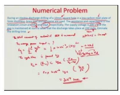
So let us actually like to, let us actually try to have numerically oriented problem where we will estimate the total machining time, so let us say we have a circuit with known parameters which is feeling to an indium setup and there is a electrode discharge drilling that we are performing where the target is to drill at 10mm square hole in a low carbon steel plate for which this relationship holds very well, the Q and W relationship that we showed in the past slide.
