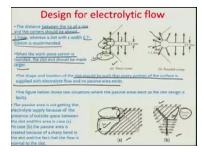
So there are several designs that has been illustrated here you can see this design as well as design B and what we are going to find out is that there are many aspects of both the designs here one is that the tune also getting loaded be by same process one is remember that there is always a minimum dimension that is needed between a slot and the end of the tool so that there is no leakage or there is no machining of the slot all the way to the edge.
