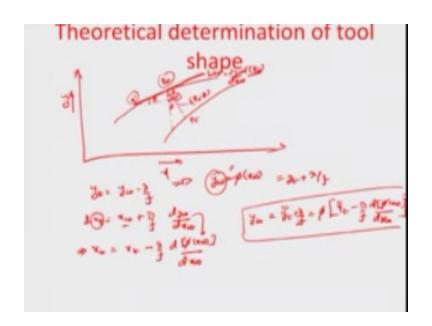
I can you know show you a little more detail just to understand this slope concept which may be you know from the geometrical idea it can come out so this is the work piece surface in the tool surface these are the two opposite points pw and PT which are connected and they are perpendicular to each other and I am talking about the feed direction the in which this particular work piece moves towards the tool surface.
