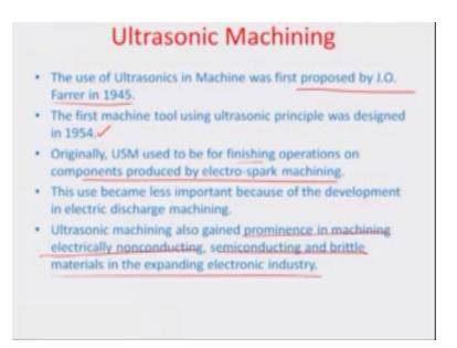
So the process was first proposed by this guy J.O. Farrer in 1945 and the first machine tool are using this USM principle or ultrasonic principle was designed about 9 years later in 1954 and originally it was used for finishing process particularly for those components which should be otherwise used by electro-spark machining or electro discharge machining.
