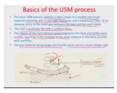
So it is basically involves tools which is otherwise ductile and tough you can see this tool right here ductile and tough tool which has a speed force and there is a slurry which is injected in to the web zone at certain pressure so the idea is the tool moves against of the slurry to the work piece so the ploughing the individual abrasive grains into the work piece.
