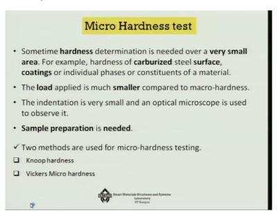
Now sometimes what happens is that this hardness is insufficient particularly when you will see that you make a very thin layer okay. So this kind of general hardness is good for when you have a single material. But many a times what happens is that we give a special surface coating on metals, okay. Let us say, when we actually work on things like suppose gears okay.
