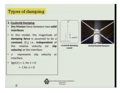
There is another type of a damping model also that is known as the Coulomb damping model, so which is basically dry friction force between 2 solid interfaces. Now in this model the magnitude of damping force unlike the last result is proportional to velocity, which means higher the velocity more is the resistance, in this case the damping force is assumed to be constant and that is it is independent of the relative velocity unlike the last case.
