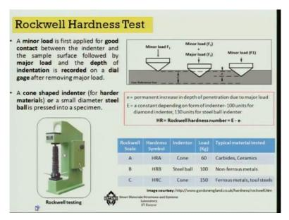
So the 1<sup>st</sup> one is the Rockwell hardness test. Now, the basic principle as I told you that resistance to plastic deformation that is same in all the cases, so only thing is that what kind of indenter you are using in terms of like this indenter if you look at it, the geometry of the indenter that actually varies from test to test.
