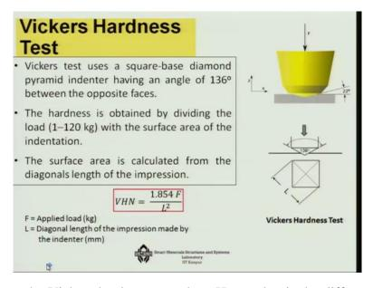
Now, we come to the Vickers hardness test okay. Here, what is the difference? Unlike this Brinell hardness test, the shape is different here as you can see that it is a square base diamond pyramid indenter and which is generally having an angle of 136 degree is between the opposite phases that is what is used in the Vickers hardness test okay. And in this case, the hardness is obtained by dividing the load which is generally 1 to 120 kg with the surface area of the indentation.
