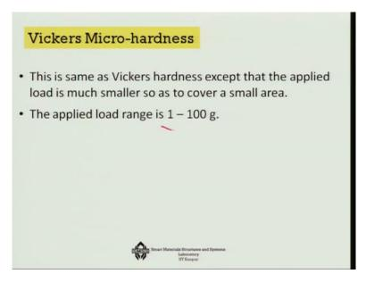
Here also you can see that the load range is 100g okay, 1 to 100 g. So that is the kind of a thing we are talking about when we talk about micro hardness test.
