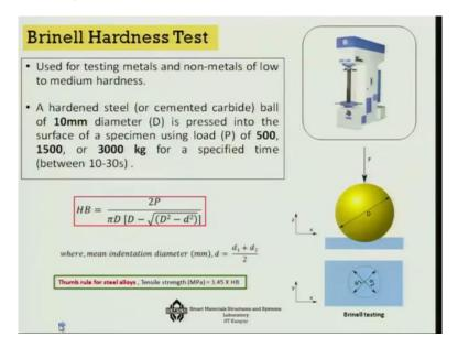
Now the other one that is also very popular is called the Brinell hardness testing. And this is used for also testing metals and nonmetals of low to medium hardness okay. So Rockwell hardness includes the ceramics also, whereas in this case it is most preferred metals and nonmetals of low to medium hardness. Now in this case however, the indentation is done not by cone, but by hardened steel ball as you can see it here by a hardened steel ball okay.
