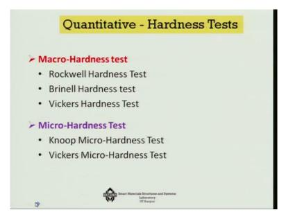
At a later stage, you know the quantitative hardness test started to get evolve and then there are basically 2 classifications of them, one is called the Macro hardness test where as I told you that not much of sample preparation is needed and the other group is called the Micro hardness test. Now in the Macro hardness there is there are many, but we have chosen Rockwell hardness test, Brinell hardness test and Vickers hardness test.
