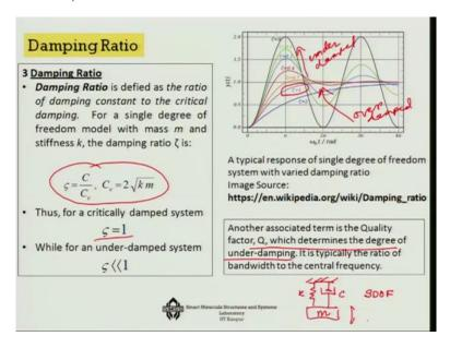
One important thing here is that what is the damping ratio? A damping ratio is basically the ratio of damping constant to the critical damping of a system. Suppose we consider a single degree of freedom system something like if you can draw it a single degree of freedom system, something like a spring here, a damper or a dashpot here and a must M okay, so this is called a single degree of freedom system, it can actually move only in one direction okay.
