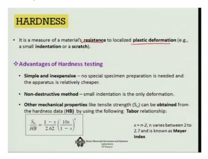
So for example, a small indentation or a scratch, so let me repeat so it is a measure of material resistance to localised plastic deformation example, a small indentation or a scratch. Now there are various advantages of hardness testing. 1<sup>st</sup> of all, it is a very simple and inexpensive test; it will not need a very special sample preparation. Of course for Micro hardness you will need, which we will talk about it subsequently.
