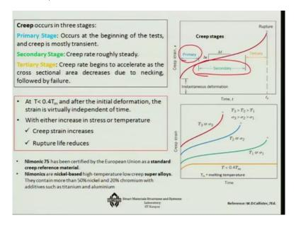
So you can get a slope, a continuous slope more or less at this stage okay and you can predict that how much it will be creeping in that time period. Then there is a tertiary stage okay, so that is you can see here with respect to time, beyond a particular time the creep increases actually exponentially as you can see in this picture. So that is you know that actually goes towards the failure.
