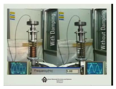
And which is typically the ratio of the bandwidth to the central frequency of the system. In the next slide I will just show you that how the damping changes the response of a system. So if you just look at this, that there are 2 systems I have shown here 1 is this is a system which is like a system which has a damper, it is like a damper which is in the form of a copper block here, which actually converts the oscillator motion inside the copper block there are actually magnetic blocks there.
