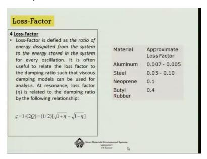
So while quantifying the damping, we have to talk about another very important factor which is known as the loss factor okay. And the loss factor is actually um defined in terms of the ratio of the energy dissipated from the system to the energy stored in the system for every oscillation, so that means you know if you consider that there is a under damped situation that means with respect to time, if you plot the response than the sponsor is in a cyclic manner.
