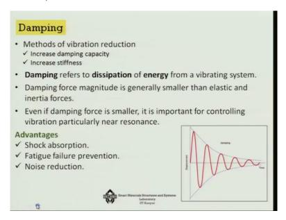
And also civil structures like which undergoes dynamic loading because of different reasons like a when loading or earthquake or maybe you know vehicles moving transport load, etc, so vibration is evacuated. Now there must be a material property which actually determines that what the level of vibration is or what is the kind of energy dissipation possible in the system.
