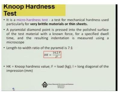
So in the Knoop hardness test, it is mostly used for very brittle materials on thin sheets okay. So here you use a pyramidal diamond point, okay which is pressed into the polished surface of the test material for a specified dwell time and the resulting indentation is measured using a microscope okay. So the length to width ratio of the pyramid is maintained as, 7 is to 1 okay.
