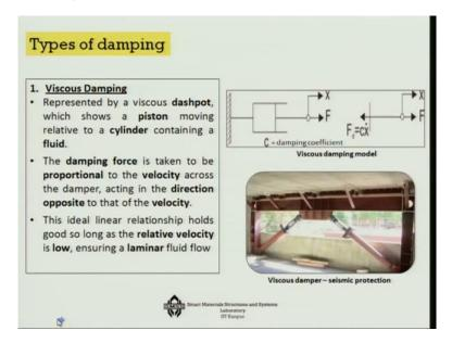
Now there are 2 important types of damping, one is called the Viscous damping and as you can see that like a seismic protection or in any door you will see that the door closer is actually a dashpot okay. So this dashpot is having actually a piston and a cylinder combination in the damping force here is considered to be proportional to the velocity across the damper acting in the direction opposite to that of the velocity.
